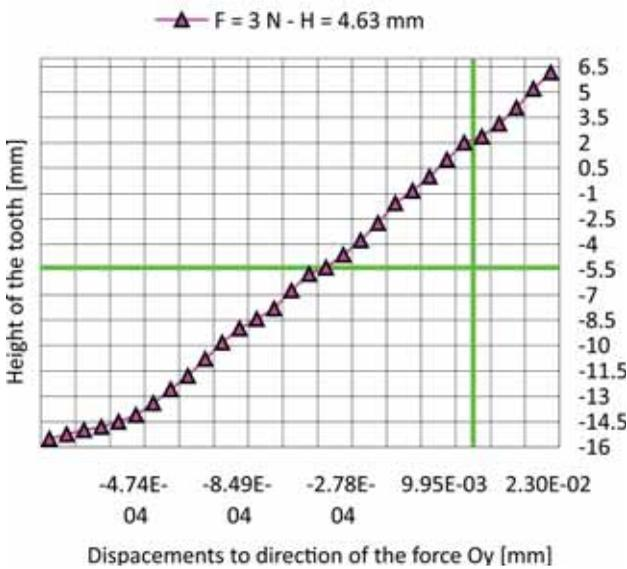
FIGURE 8. Position of the center of rotation  $C_{rot}$  for the position of the bracket  $H = 4.63 \text{ mm}$  and loading with  $F = 3 \text{ N}$
